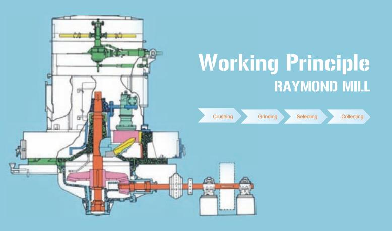
Firstly, raw material is crushed by jaw crusher to the size required, then the crushed materials are elevated into a hopper from which the material is transported through the electro-magnetic vibrating feeder, evenly and continuously into the grinding chamber for powder-processing. The rollers oscillate outward to press the ring because of the centrifugal force and the shovel scoops up the materials, send to the middle between ring and roller to accomplish the grind.
